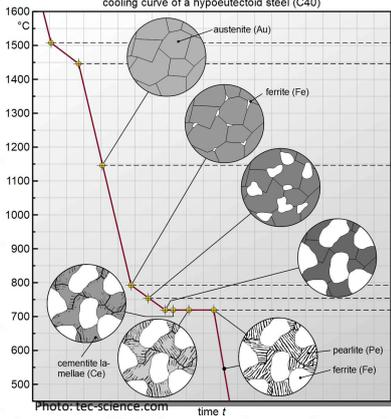
cooling curve of a hypoeutectoid steel (C40)
