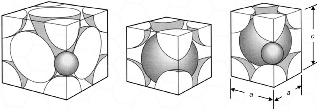
BCT is inherent metastable: meaning C will diffuse from the Octahedral space, when heated.
