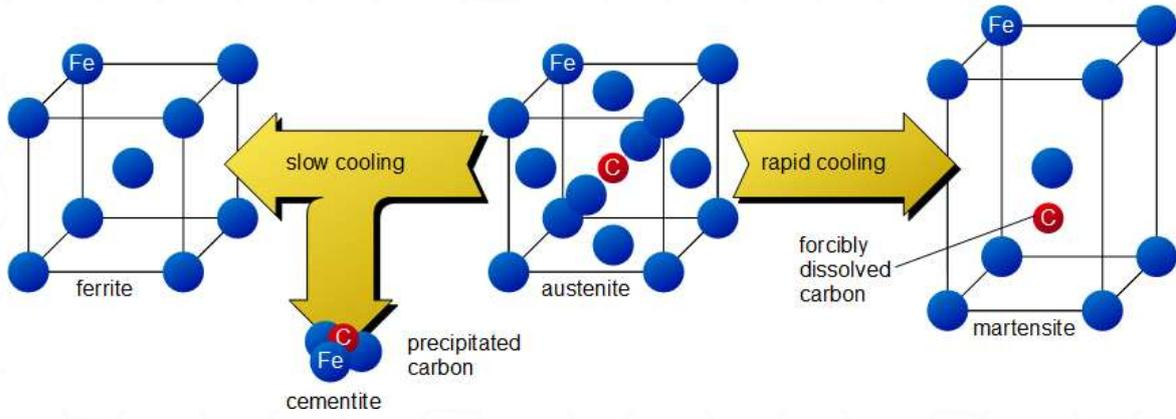
The diagram illustrates the phase transformation of austenite (Fe-C) under different cooling conditions:
