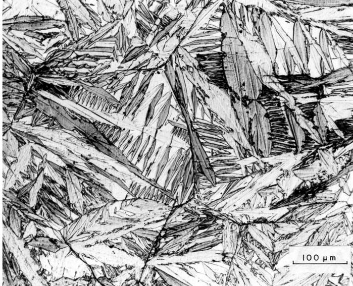
When >1,0% Carbon, Martensite will be shaped in Lenticular discs, the 'classic' needle shaped structure we (most likely) all recognize.
