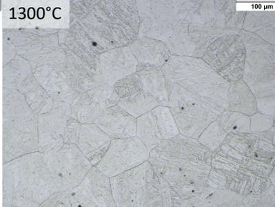
For determining the relation between Prior Austenite Grain Size (PAGS) and  $M_S$  and  $M_F$ , the steel was transformed to Austenite for 180 sec and cooled.
