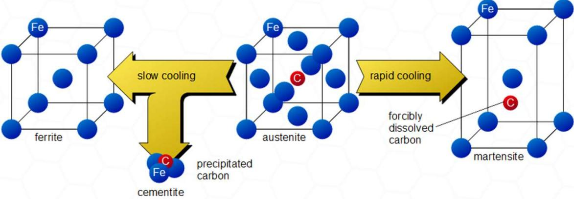
The diagram illustrates the phase transformations of steel based on cooling rate. It starts with austenite (Fe lattice with interstitial C atoms).
