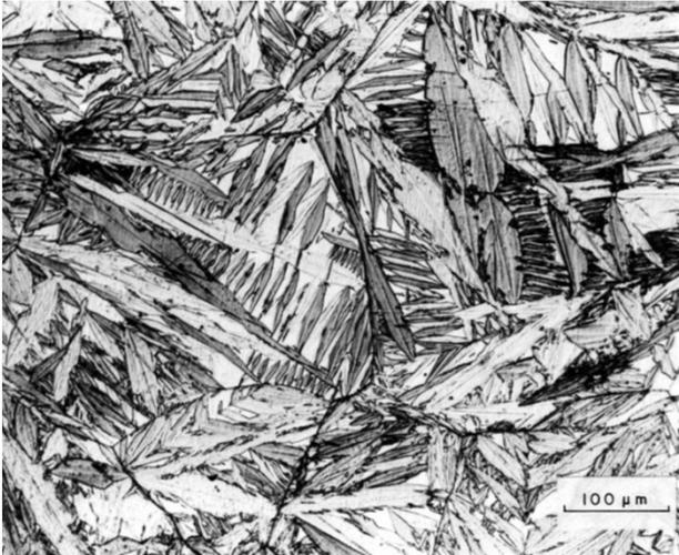
A 'typical' picture of Martensite **in steel** we all can recognize.
